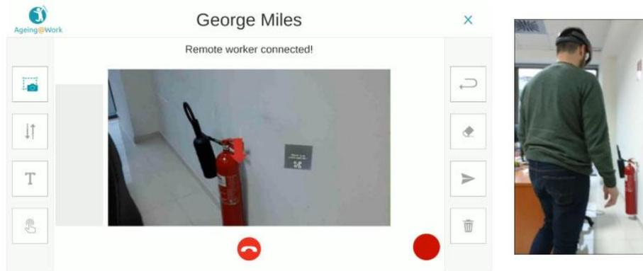
**Fig. 2.** Remote supervisor app view with live stream from the Hololens camera (left) On-site worker wearing the Hololens (right)
